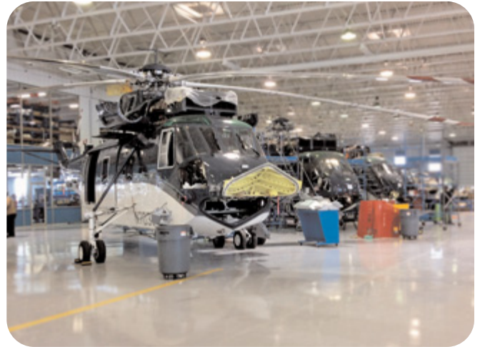
S-61 Helicopters in various stages of restoration
