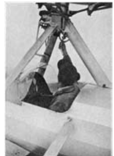
Pilot pulls lever as shown, to convert ship from one type to the other. Balance mechanism allows lever starts rotating freely. Locking mechanism for speed flight is nearly simple.
